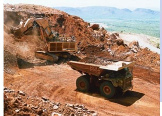
*Over 22 million tons of barren overburden had to be removed to expose the Argyle pipe.*
