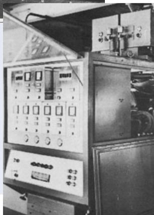
In modern treatment plants, an x-ray separator is used. As diamonds pass through the x-ray beam, they trigger an airjet, which blows them into a container.
