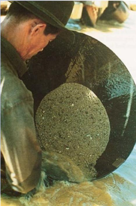
*The age-old technique of panning is still used to recover diamonds from some alluvial deposits.*
