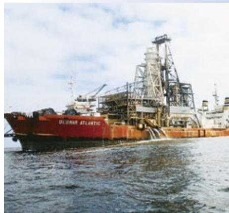
*Marine deposits are as far as 60 miles from shore in water as deep as 500 feet. Marine mining technology involves sophisticated vacuum systems for sucking up diamond bearing sediment from the ocean floor.*
