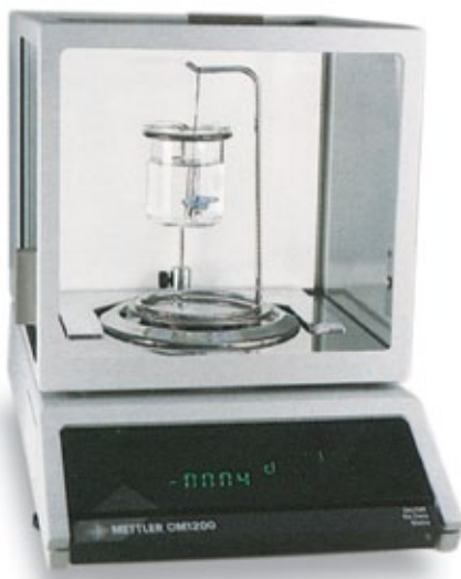
Today, most jewelers use electronic balances. They are simple, fast, and most are accurate to a tenth of a point (0.001 ct.).
